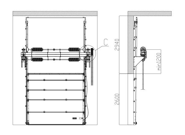
Additional parameters of the opening when using a chain drive of type CH0501.
